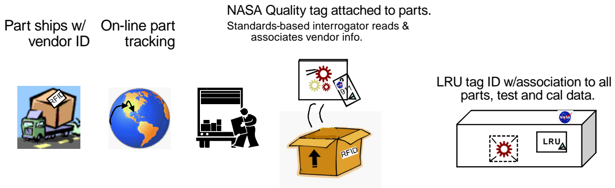
Figure 3-3: RFID Ground-to-Line Replacement Unit Concept
