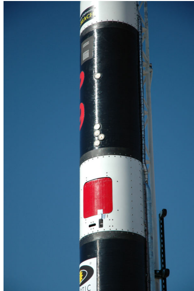
Figure D-12: Passive Temperature RFID/Sensor Tags on Rocket Fuel Tank
