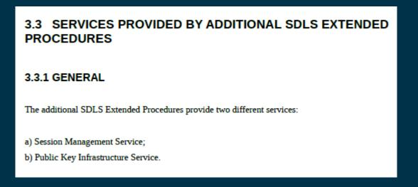
Session Management Services based on Elliptic Curve Diffie-Hellmann (ECDH) for key exchange. Edwards-curve Digital Signature algorithm for authentication and identity verification (EdDSA)
