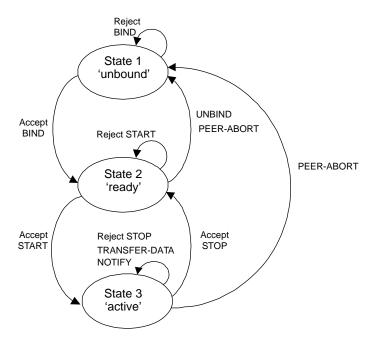
Figure 7-4: Example State Machine Diagram—SLE RCF
