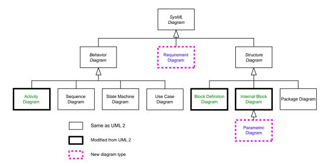
Figure B-1: SysML Diagram Types (SysML Partners)
