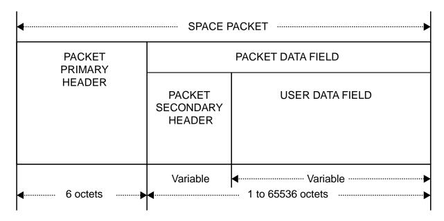
Figure 7-3: PDU Example, Space Packet Protocol
